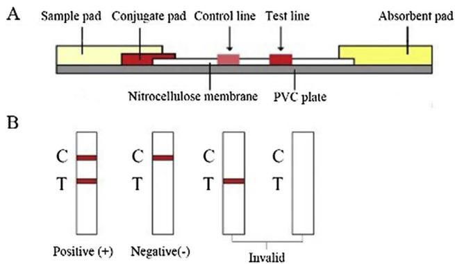
Fig. 1. The composition of the immunochromatographic test strip. (A) The Schematic Description of the Immunochromatographic Device. (B) The Illustration of Immunochromatographic Test Results.
